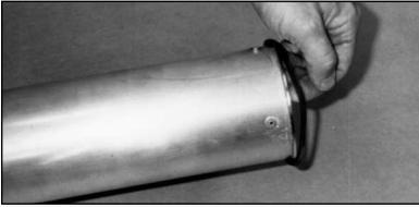
**Step 15:** Install the o-ring (p/n 561683, supplied).
