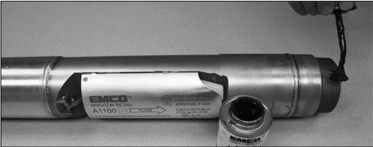
**Step 16:** Apply a liberal coat of pipe dope to male threads of the A1100 base.
