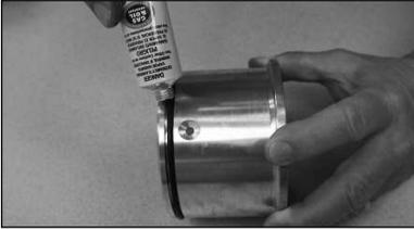
**Step 11:** Remove the top o-ring from the collar, if in place. Apply a heavy coat of the sealant (p/n 566726, supplied) around the O-ring and a light coat inside the tube. Make sure the O-ring (p/n 480049, supplied) is installed in the groove of the collar.
