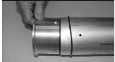
**Step 12:** Place the loose o-ring onto outside of drop tube. Slide adaptor inside top of drop tube and up tight to the drop tube adapter flange. This will be a tight fit. If necessary, use a wood block across the adaptor to tap into place. Align the 4 holes. Slide top o-ring into place.
