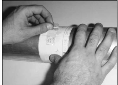
**Step 6:** Wrap the paper drilling template (p/n 566710S, supplied) over the drop tube and tape in place. Line up cut-off line on template with the cut length C.
