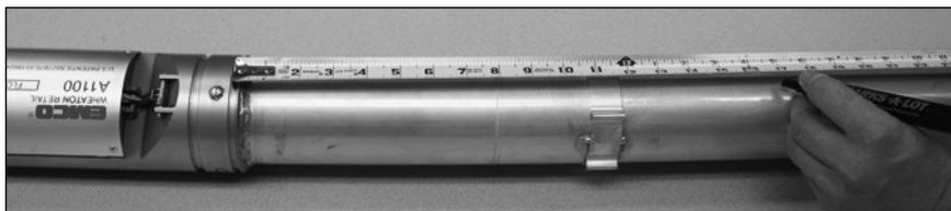
**Step 5:** Measure length C from the bottom of top tube.
