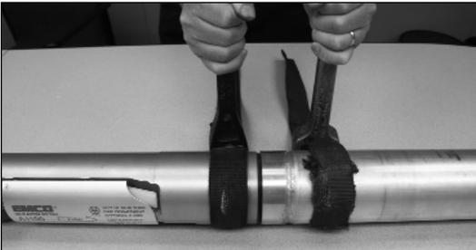
**Step 15:** Tighten. The use of strap wrenches is recommended in order to prevent raising burrs on the aluminum parts.
