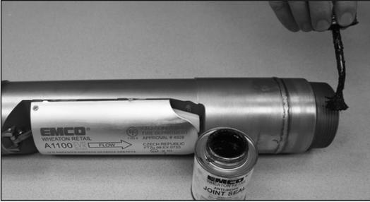
**Step 13:** Apply a liberal coat of pipe dope to male threads of the A1100 base.
